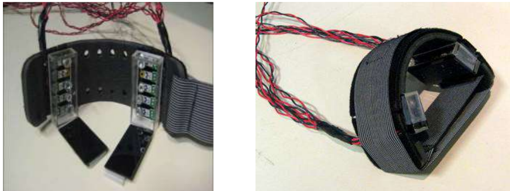
Figure 5. A wearable, bio-acoustic sensing array built into an armband and prototype armband.
