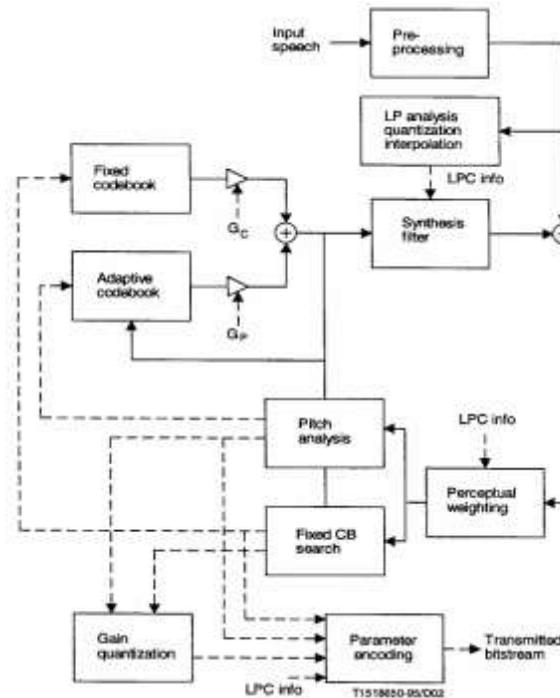
Fig-[4], Block diagram of ACELP encoder [12]
