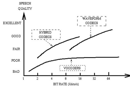
Fig. [1], the speech quality mean opinion score for various bit rates [10]
