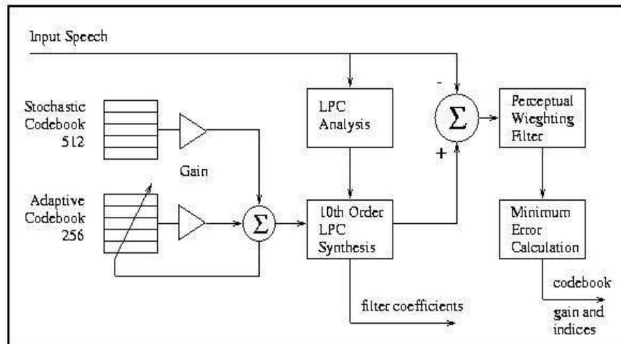
Fig-[2], Block diagram of CELP encoder [12]
