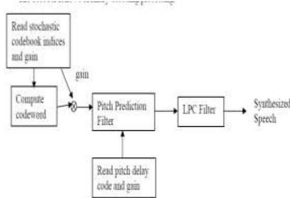
Fig-[3], Block diagram of CELP decoder [12]
