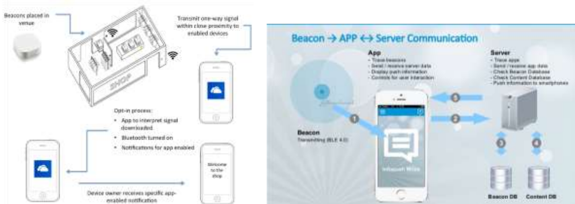
Fig: 1 Beacon Work Model [5]
