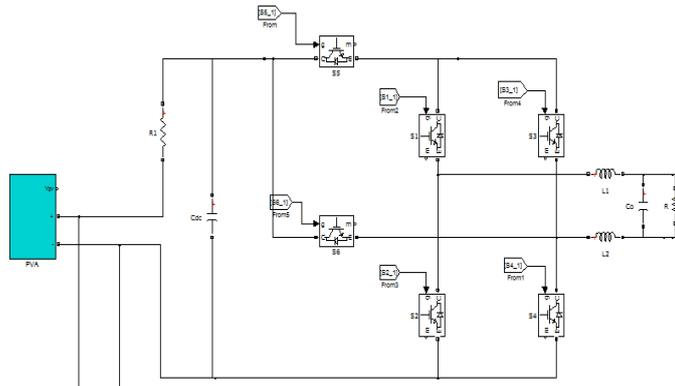
Figure 15. Proposed H6 Simulink Model with attached PVA
