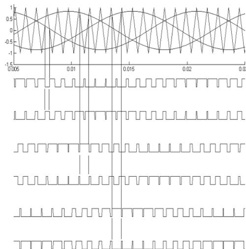
**Figure 5. Generation of Pulses with respect to Reference Fundamental Waveforms**
