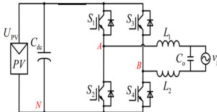
**Figure 1. Conventional Four Switch Inverter**
