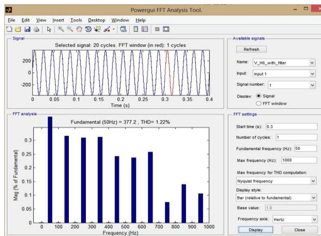
Figure 16. FFT Analysis of Phase-A Voltage ( $V_A$ )
