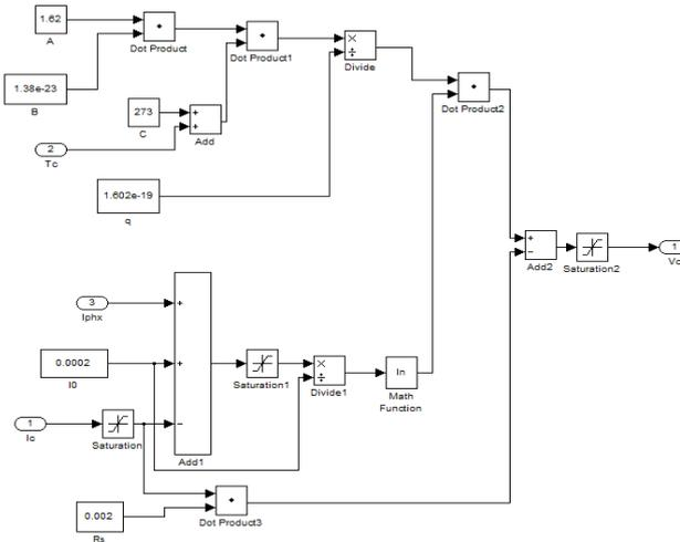
Figure 7. Simulink model of  $V_c$
