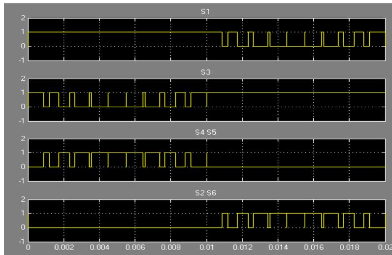
Figure 16. Pulse Waveforms of S1-S6 Switches for H6 Topology Simulink
