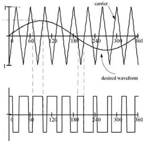
**Figure 1. PWM Scheme for Conventional Inverter**
