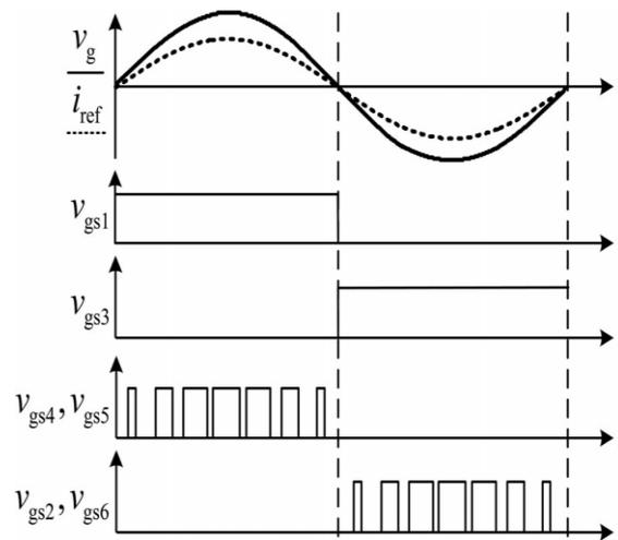
*Figure 14. PWM Gate Signals for Switches S1-S6 of Proposed H6 Topology*
