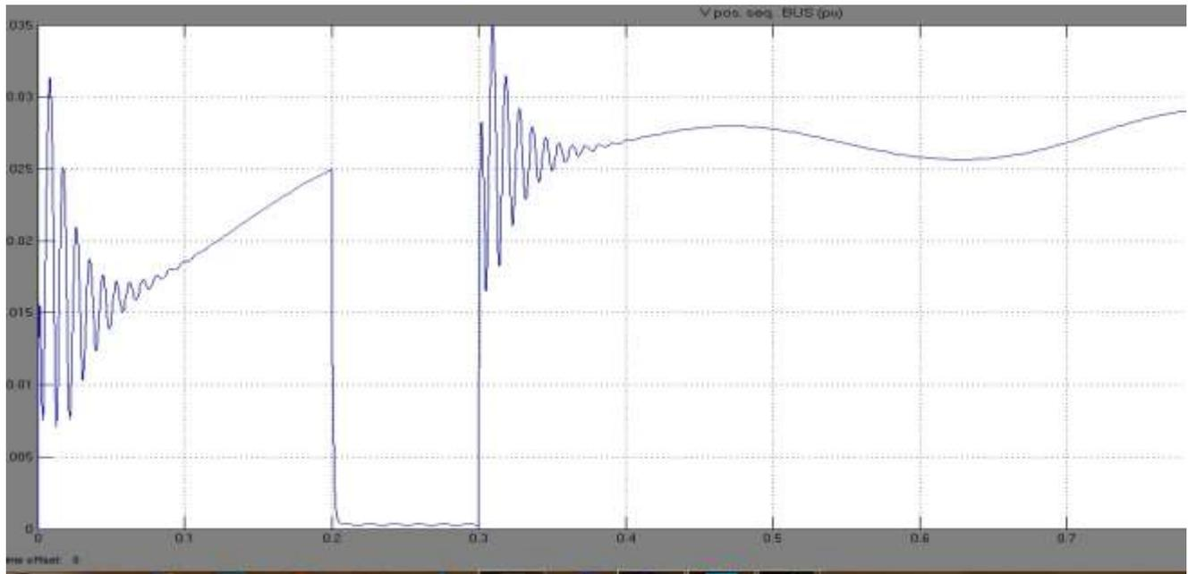
Fig.8. SMIB Waveform Of Voltage P.u V/S Time (LG Fault) with SVC
