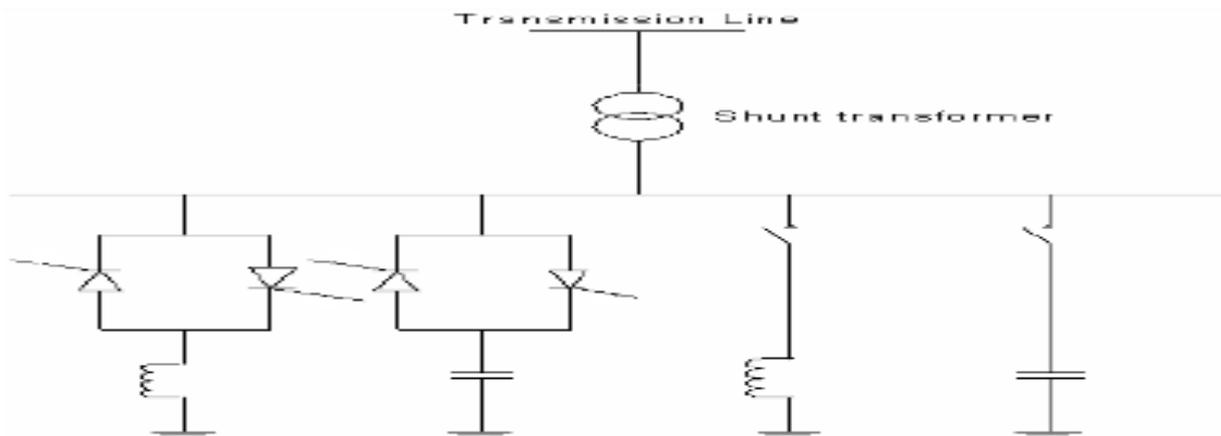
Fig.3. Single Line Diagram of SVC[18]
