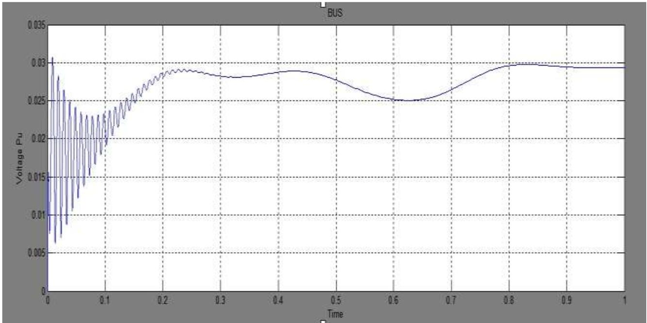
Fig.6.SMIB Waveform Of Voltage P.u V/S Time (During Normal Condition) without SVC
