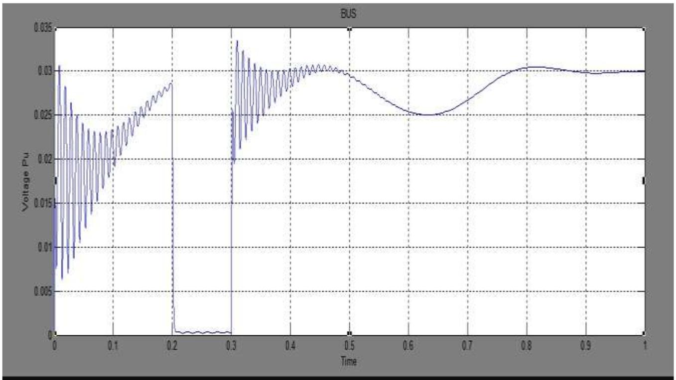
Fig.7.SMIB Waveform Of Voltage P.u V/S Time (LG Fault) without SVC
