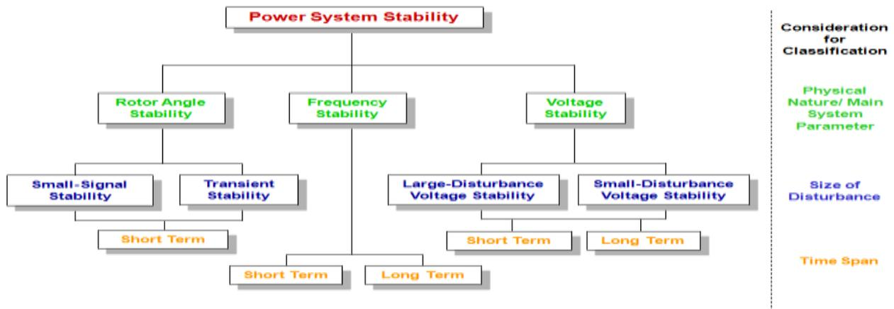
Fig.1 Classification of Power System Stability[1]
