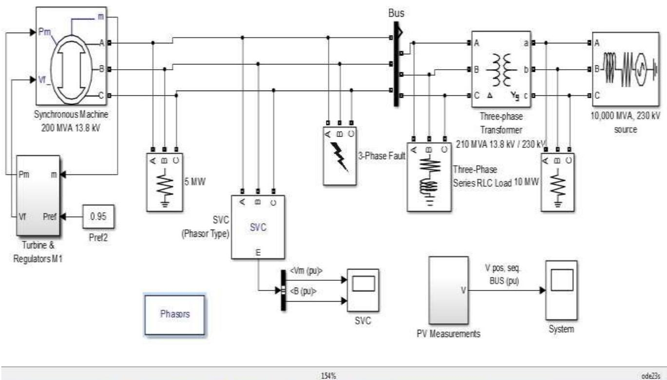
Fig.5. Single machine infinite bus bar Model
