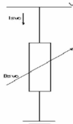
Fig.4. Equivalent Circuit Diagram of SVC [8]
