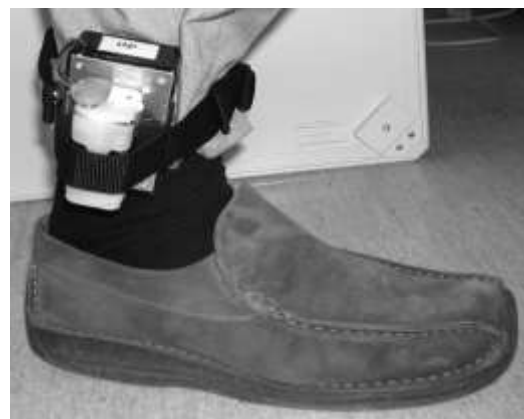
Figure 4: The MR sensor attached to the lower leg
