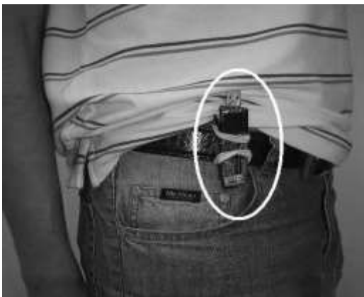
Figure 3: The MR sensor attached to the hip from [1]
