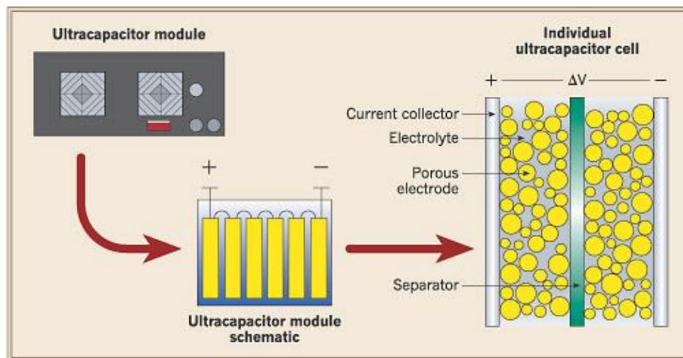
**Fig. 1** Ultracapacitor Module
