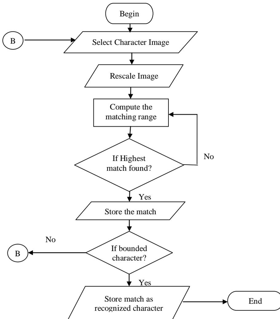
Figure 3. Flowchart for implementation of Template Matching for OCR
